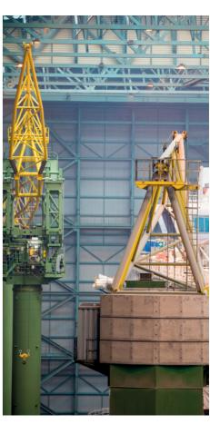
A new 16 tonne crane called "Mangokautz" has been operating in hall 6 since the start of the year. The new crane has an adjustable jib, giving it roughly 10 metres more lift than our other arm cranes. This is important in view of the fact that components are getting higher and higher. Therefore in hall 6, crane operations are now possible up to deck 20 and 60 cm below the roof.
